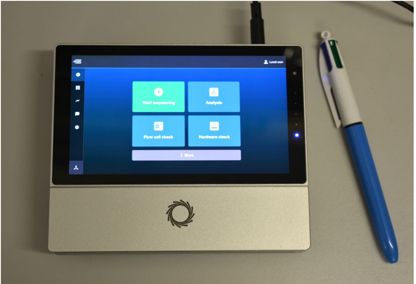
The nanopore DNA sequencing device. Photograph credit: Nga Tran
